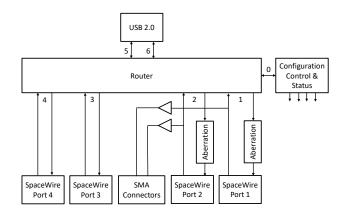
The SPLT has two normal SpaceWire interfaces (ports 3 & 4) and two SpaceWire interfaces where the LVDS transmit signals can be altered to support physical layer margin testing (ports 1 & 2). Special aberration circuitry is able to adjust the in-pair and data-strobe skew, change the signal amplitude and adjust the common-mode voltage. Aberrations are made under control of software running on a host computer via the USB 2.0 port and the configuration, control and status circuitry.
