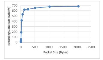
Packet Size vs Aggregate Recording Data Rate
