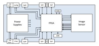
Figure 2: SpaceFibre Camera Block Diagram
