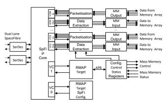
Figure 4: Dual-Lane SpaceFibre Mass-Memory Interface
