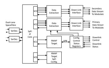
Figure 6: Dual-Lane SpaceFibre Downlink Interface
