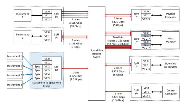
Figure 8: Example SpaceFibre Payload Data-Handling Network
