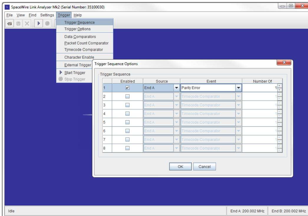
**Trigger on Parity Error**
