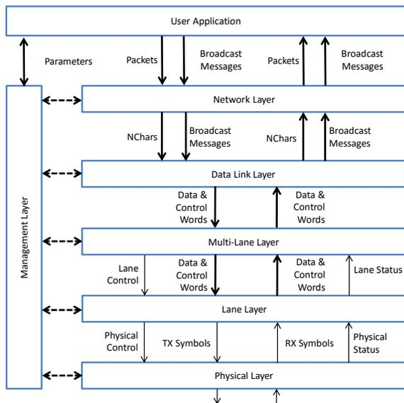
**Fig. 1 SpaceFibre Protocol Stack**
