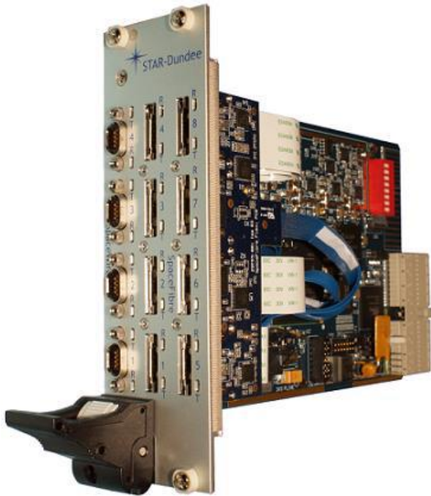
Figure 3 SUNRISE SpaceFibre Router
