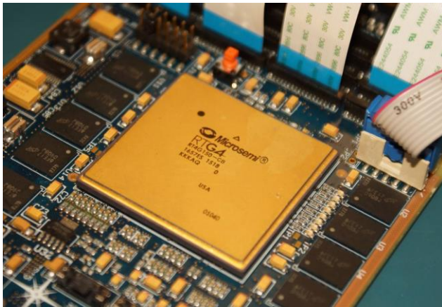
Figure 6 Prototype Microsemi RTG4 board for SUNRISE SpaceFibre Router
