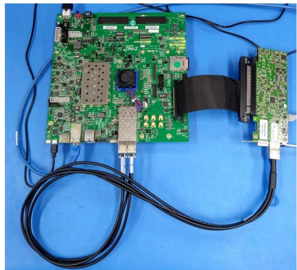
Figure 3-1: SpaceFibre Endpoint Test System
