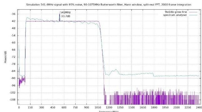
Figure 2: WBS-VIII Simulation Performance (Purple) versus a Spectrum Analyser (Green)
