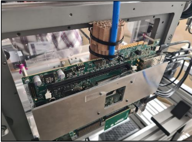
Fig. 4. Test Setup with the VCK190 board in place for radiation testing.
