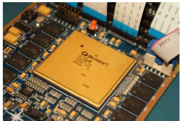
**Figure 4. Prototype board for SUNRISE SpaceFibre Routers**
