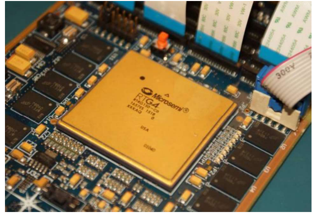
Figure 8 Prototype Microsemi RTG4 board for SUNRISE SpaceFibre Router
