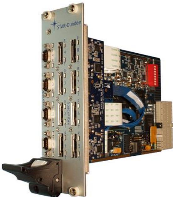
Figure 8. PXI Board configured as SpaceFibre Router
