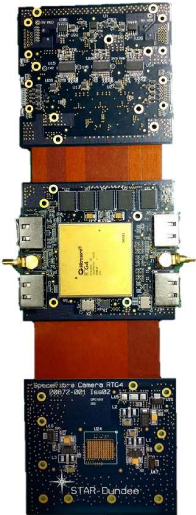
Fig. 5. Assembled SpaceFibre Camera PCB
