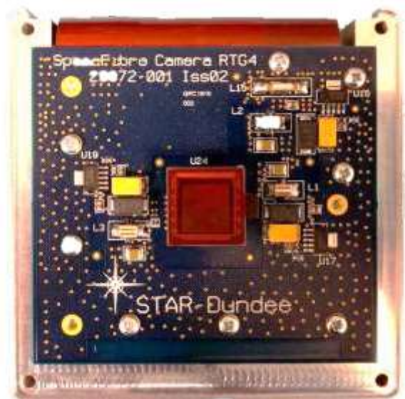
Fig. 8. SpaceFibre Camera Partly Installed in Box
