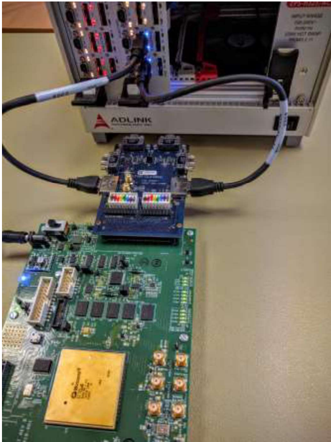
Fig. 4. SpFi Multi-Lane IP interconnection test between RTG4 and Spartan FPGAs
