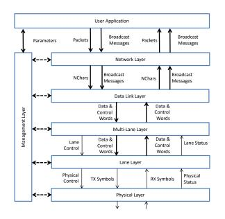
Fig. 1 SpaceFibre Protocol Stack
