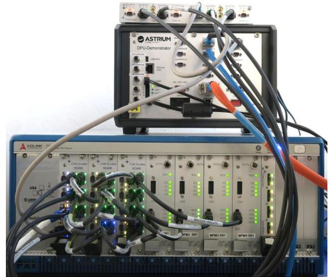
Figure 5: Prototype Next Generation Mass Memory System
