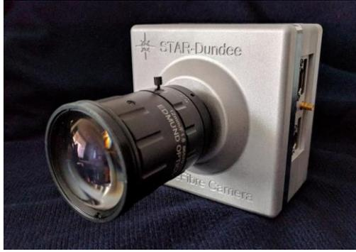
Figure 3: SpaceFibre Camera
