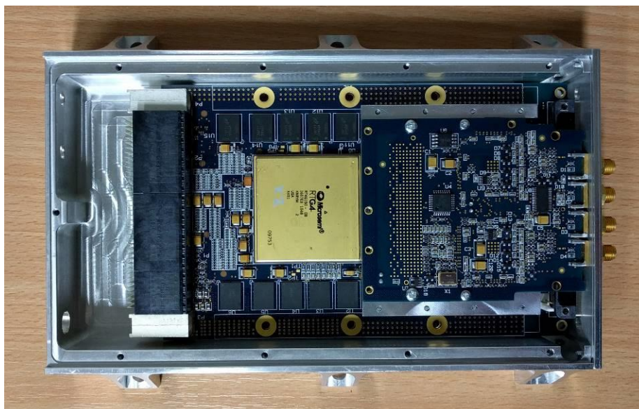
Figure 4 SpaceVPX-RTG4 Board with Dual ADC FMC card fitted
