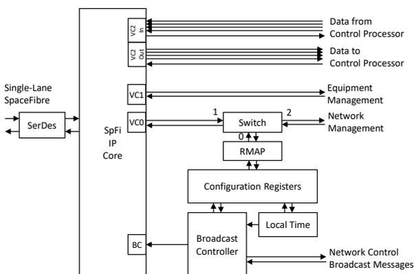
**Figure 7: SpaceFibre Control Computer Interface**
