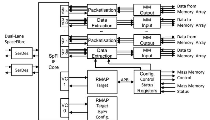
**Figure 4: Dual-Lane SpaceFibre Mass-Memory Interface**
