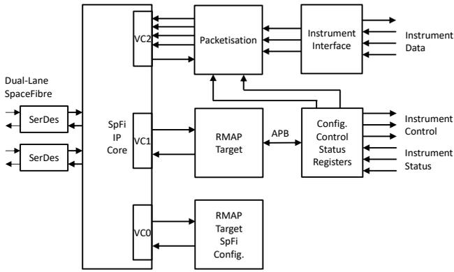
**Figure 2: Dual-Lane SpaceFibre Instrument Interface**
