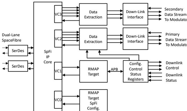
**Figure 6: Dual-Lane SpaceFibre Downlink Interface**
