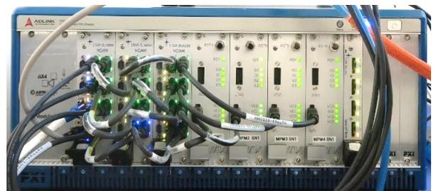
**Figure 5: Prototype Next Generation Mass Memory System**
