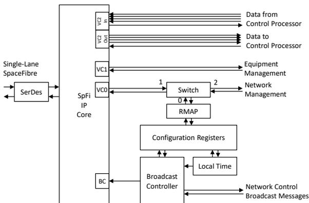
**Figure 7: SpaceFibre Control Computer Interface**
