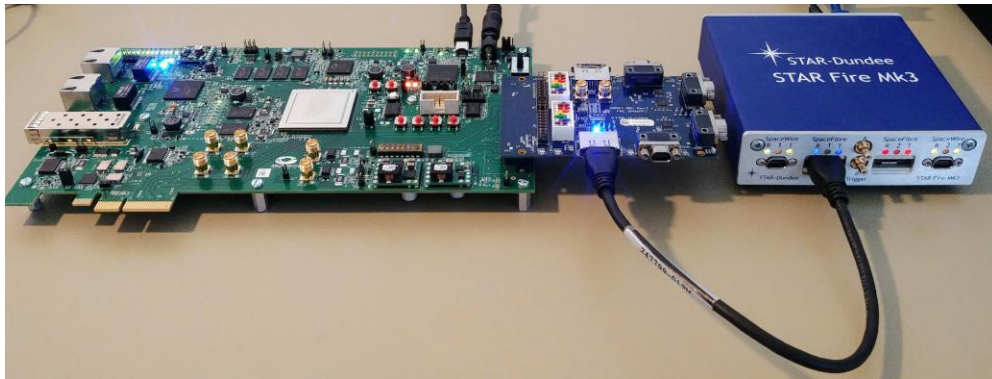
Figure 1: SpaceFibre running on a PolarFire FPGA and connected to the STAR Fire Mk3 EGSE
