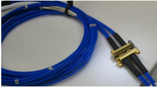
Fig. 8. Prototype SpaceFibre Flight Cable from Axon
