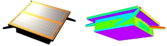
PANGU PRISMA/Tango model (left) and false colour temperature (right)
