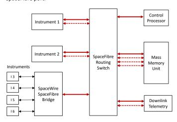
The control processor is used to configure and control all on-board data-handling equipment. It therefore needs a connection to every instrument and to the mass memory. This could be provided using a separate command and control network, but it would result in additional mass and power consumption. The addition of a SpaceFibre router connected to all of the on-board equipment allows the control processor to send commands and receive information from all of the on-board data handling units.
