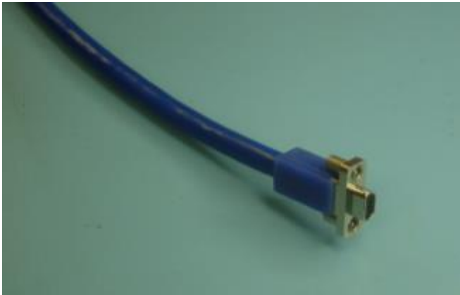
Figure 1: Innovative Connector Assembly on SpaceWire Lab Cable
